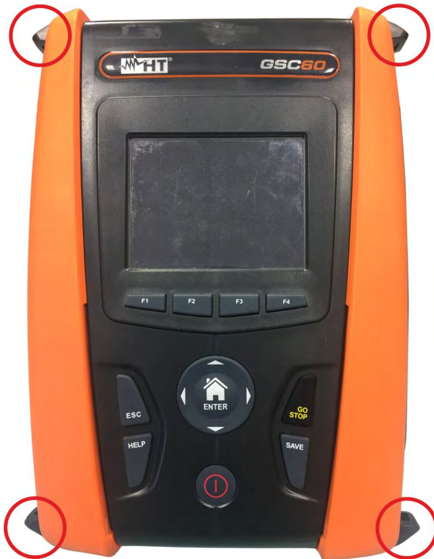
Fig. 48: Instrument with fitted half-shells and hooks
