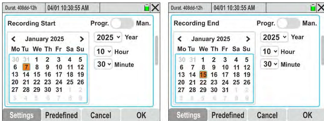
Fig. 30: Setting the programmed recording Start/End date
