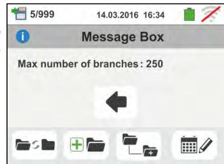
5. In case tries to include a comment of length higher than 30 chars, the instrument provides the warning screen shown to the side
