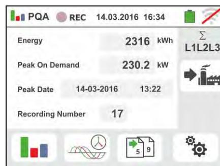
18 Touch the
