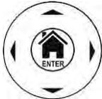
◀ ▶ ▲ ▼ keys to move the cursor through the different screens in order to select the desired programming parameters
