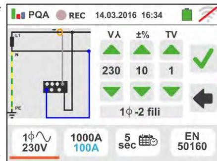
3. Move the slide bar cursor in order to select the type of clamp for phase current and neutral current measurement (marked in blue color), considering that the clamps can be of different types, between the options:
