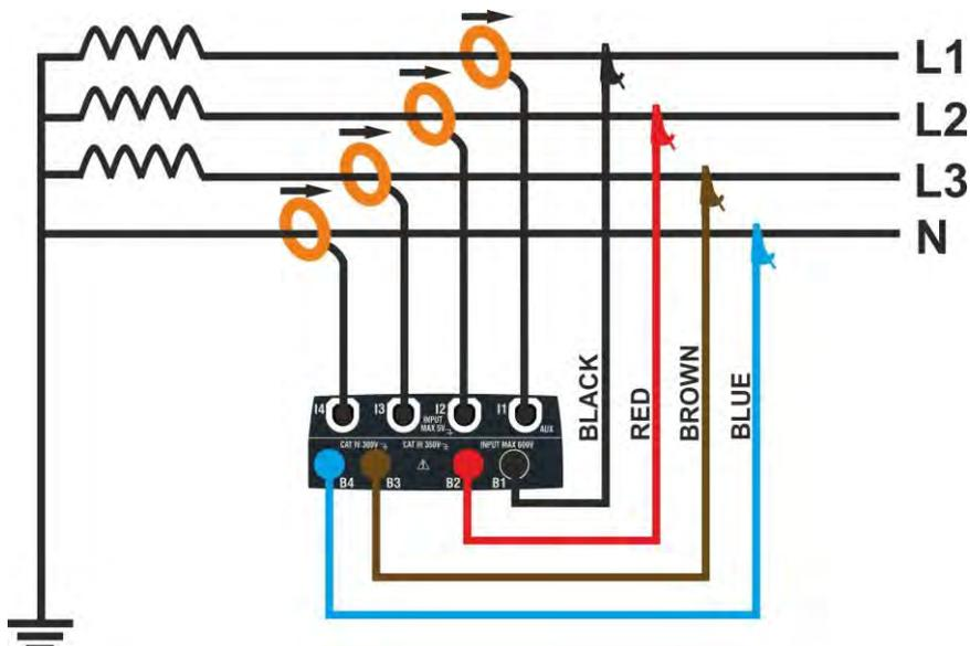
Fig. 10: Connection for measurement on Three-phase system **3φ-4WIRES**
