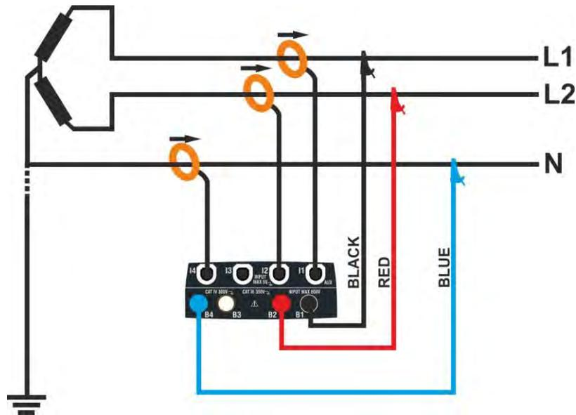
Fig. 15: Connection for measurement on Two-phase system 3-wires **3φ-Y Open**
