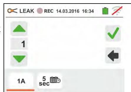
3. Move the left slide bar cursor in order to select the aggregation time (see § 12.5) among the options: **2s, 5s, 10s, 30s, 1min, 2min, 5min, 10min, 15min, 30min**
