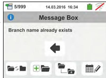
4. In case tries to define a numebr of nodes of 1st, 2nd and 3rd level higher than 250 (for each level), the instrument provides the warning screen shown to the side
