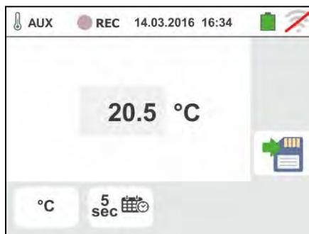
6. Press the **GO/STOP** key to start recording. The instrument enters stand-by mode (waiting for the next minute or the set date/time) and the “” symbol is displayed as shown in the screen to the side.
