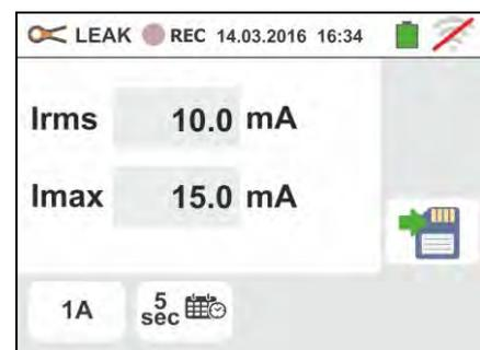
7. Press the **GO/STOP** key to start recording. The instrument enters stand-by mode (waiting for the next minute or the set date/time) and the “” symbol is displayed as shown in the screen to the side.
