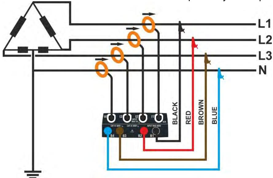
Fig. 13: Connection for measurement on Three-phase system 4-wires  $3\phi$ -High Leg
