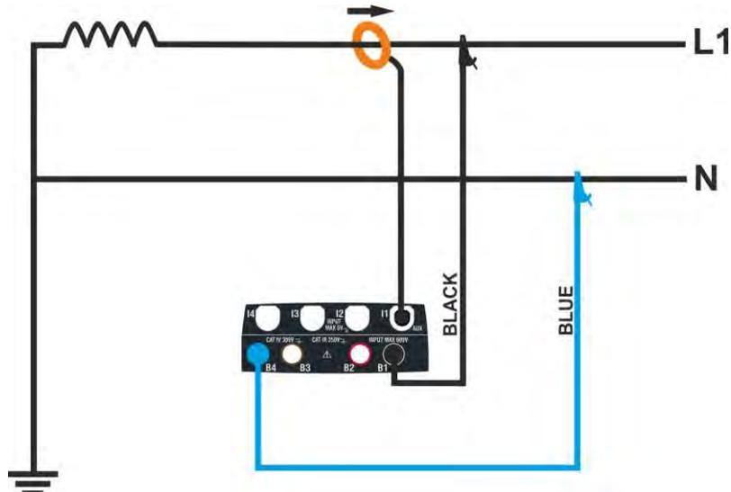
Fig. 9: Connection for measurement on single-phase **1φ-2WIRES**
