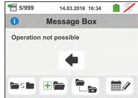
3. In case tries to create a sub-node by using a just used name, the instrument provides the warning screen shown to the side and is necessary to define a new name
