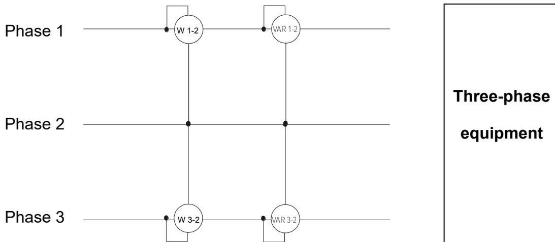
In this case the potential of one of the three phases (for example, phase 2) is taken on as reference potential. The total values of the active, reactive and apparent power are expressed as sum of the indications of the couples of Wattmeters, VARmeters and VAmeters.
