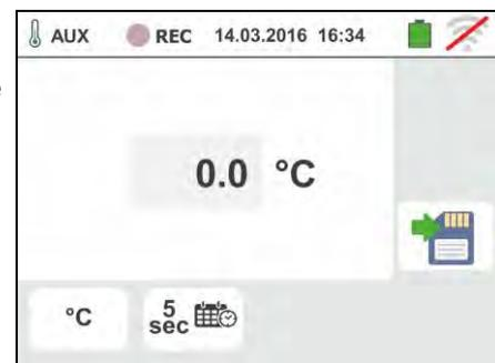
2 Move the slide bar reference to select the type of measurement among the options: °C (temperature in Celsius degrees), °F (temperature in Fahrenheit degrees), **Lux(20)** (illuminance with 20Lux capacity), **Lux(2k)** (illuminance with 2kLux capacity), **Lux(20k)** (illuminance with 20kLux capacity), **%RH** (relative humidity), **mV** (measurement of DC voltage up to 1V)
