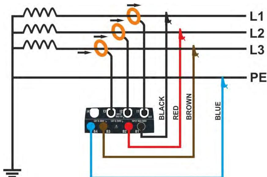
Fig. 11: Connection for measurement on Three-phase system **3φ-3WIRES**
