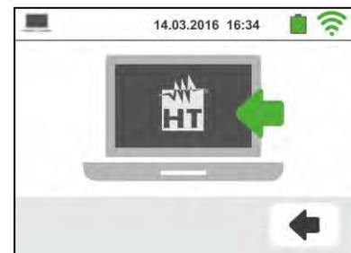
2. Enable the WiFi connection on the target PC (ex: by using a WiFi key installed and connected to a USB port) and connect to the WiFi network enabled by the instrument (name of network “VEGA74\_XXXXXX” where XXXXXX is the serial number of the instrument)
