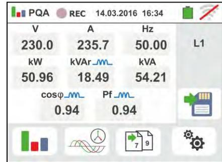
9. Touch the
