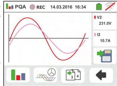
Press the **SAVE** button or touch the
