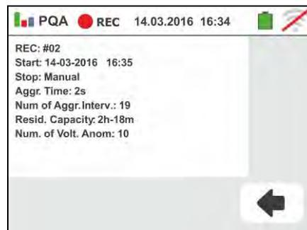
16 Press the **GO/STOP** key to stop recording; the instrument automatically saves the result in its memory (see § 7.1.3). The message to the side is shown.
