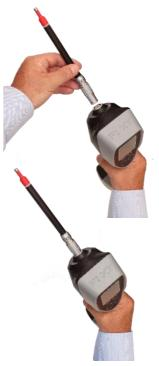
To switch the instrument **ON** press the **left button** on the Handgun shortly.
