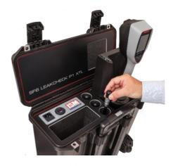
Attach the **P1 SmartSensor** into the plug at the handgun before you switch the instrument on.
