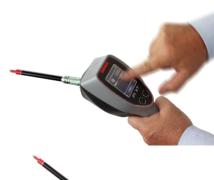
To set the measured value to **Zero** press right button shortly.
