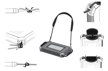
Caution: ensure all strap connections are fitted correctly and secure before use.
