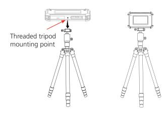
**CAUTION**: Ensure tripod and mount screws are tight and secure before use.
